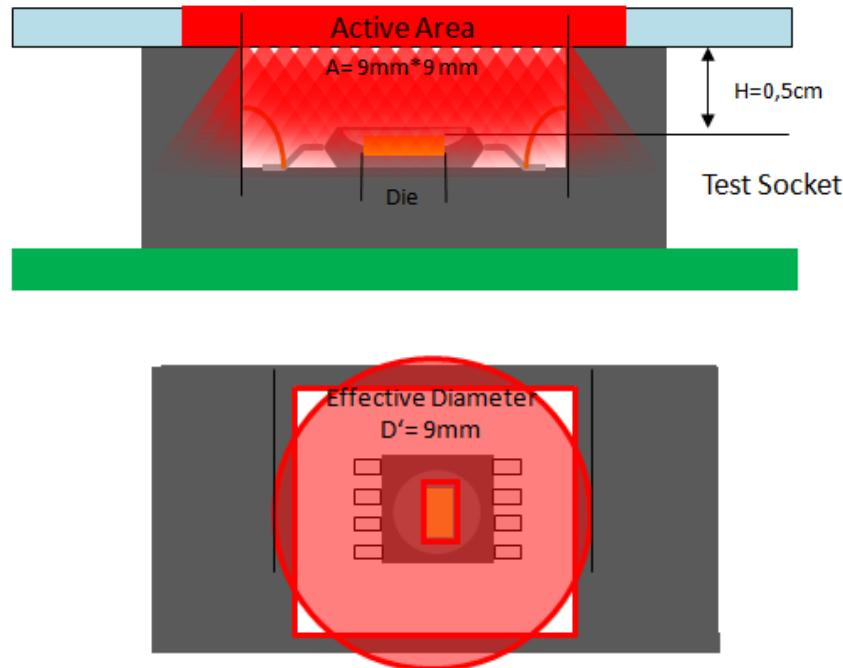
Not all alpha particles emitted from a specific point of the area (AA) will hit the die. The probability to hit the die decreases with the distance between active area and the inverse of the effective diameter of the active area. According to [13] a raw estimation for the compensation factor can be calculated by:
