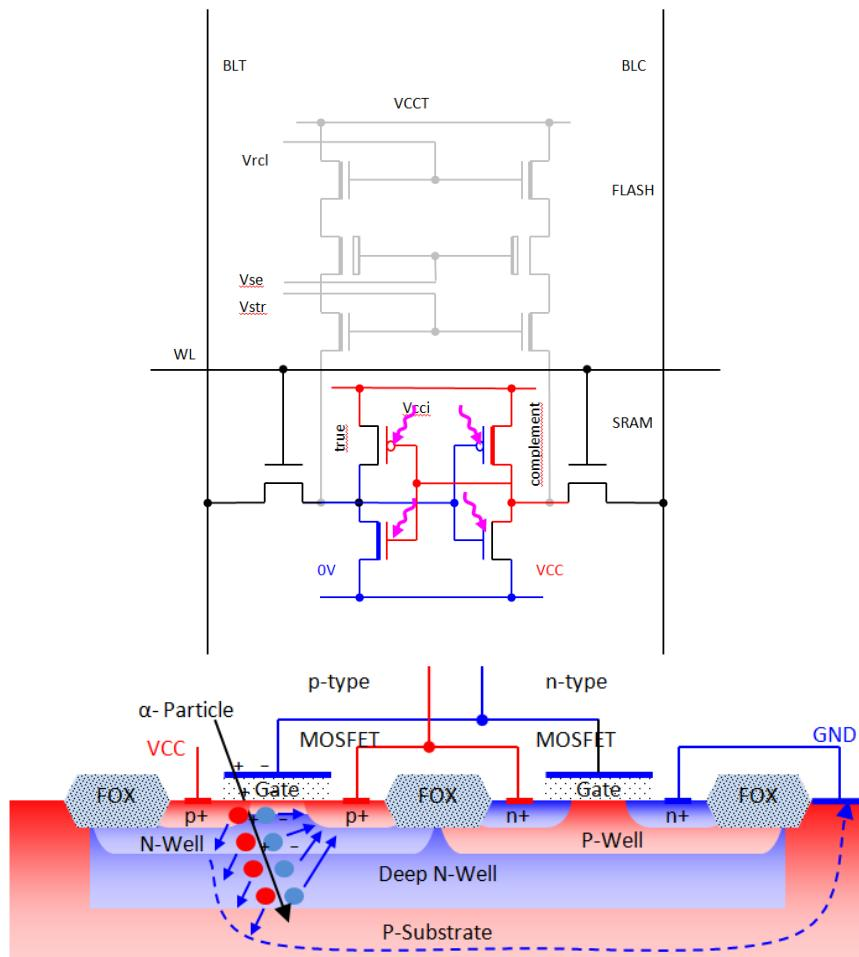
The holes drift to the substrat and the electrons drift to the nodes. If the current is too high, the SRAM cell may flip. This is called a Soft Error or single-event upset.
